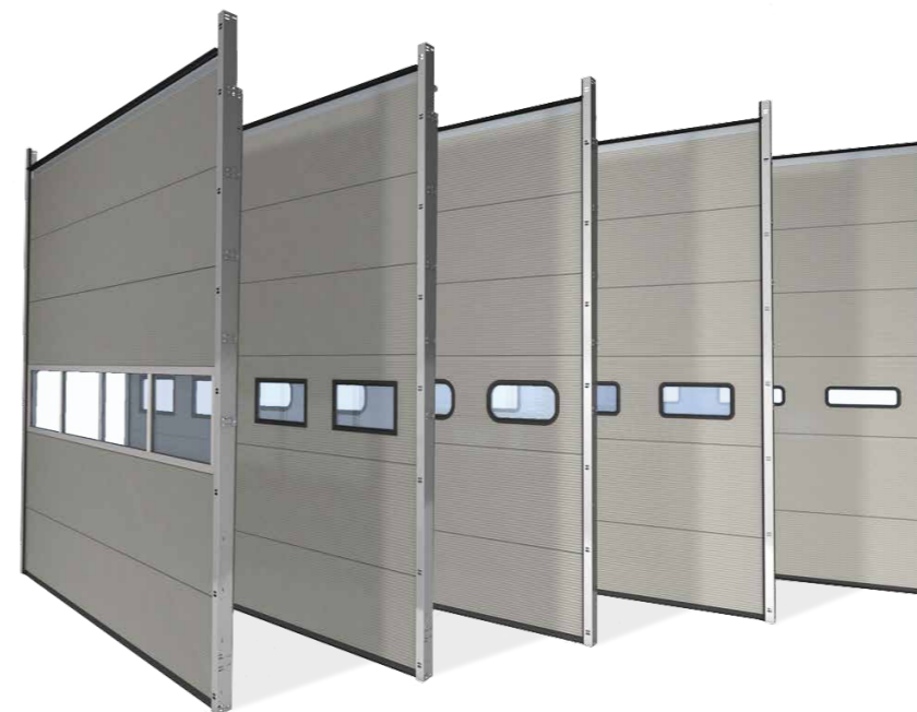
U-value ISO 40 mm sectional door: 5,000 x 5,000 mm: 1.05 W/m 2 K
